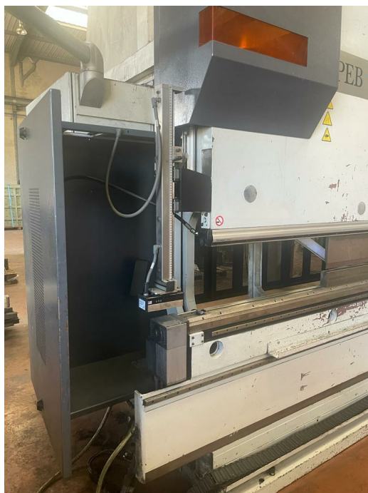
LASER - BOMBEE MOTORISE - BRIDAGES HYDRAULIQUES WILA
