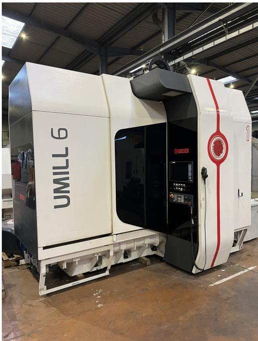
CENTRE D USINAGE VERTICAL 5 AXES HURON UMILL6
